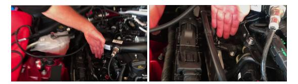
Disconnect the factory Manifold Pressure Sensor from the factory harness.
